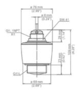
4-20 mA/0-8 m radar sensor for measuring levels without coming into contact with effluent.
