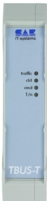
Figure 30: TBUS remote-IO with max. 10 clusters
