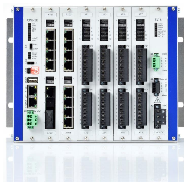
Figure 25: Example BCU-50-M-W with 4 network segments
