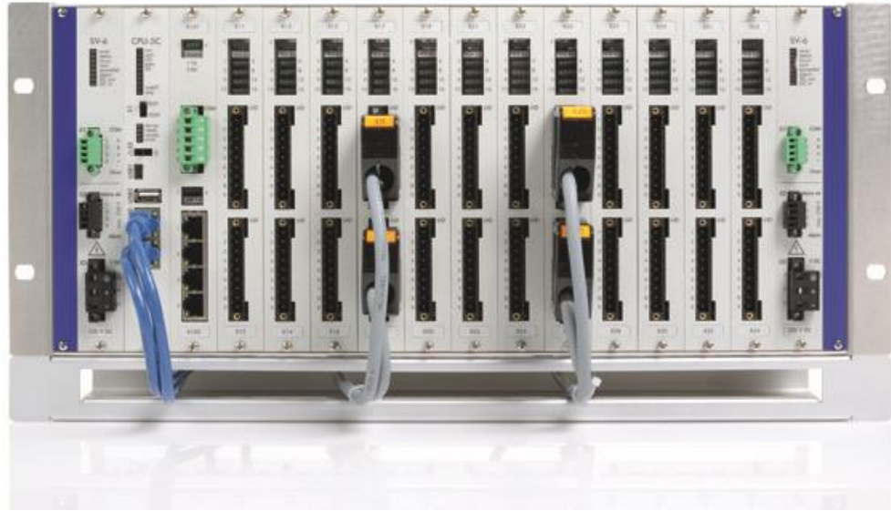
Figure 21: BCU-50 with SV-6 main supply and redundant SV-6
