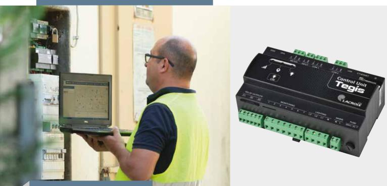
The Tegis control unit is installed in the street lighting cabinet to enable its smart management.
